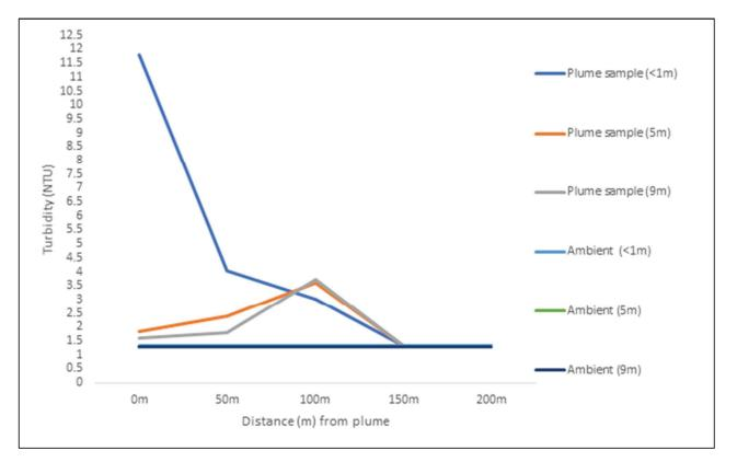
Figure 6-2: Turbidity Results at 50 m Intervals from Plume Source
