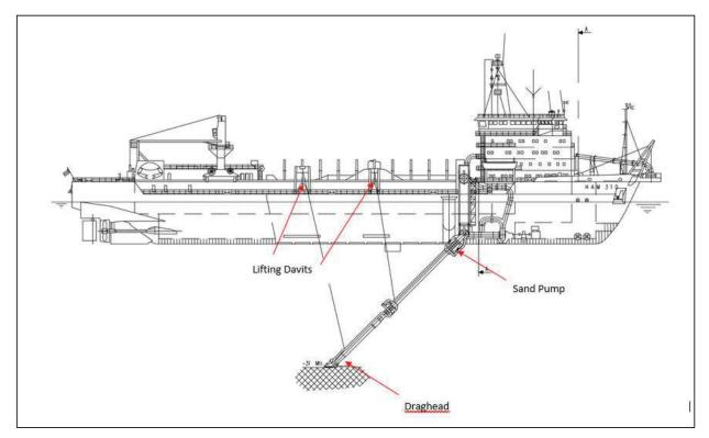
Figure 2-1: Schematic Diagram of Trailing Suction Hopper Dredge (note not an actual MBL vessel)
